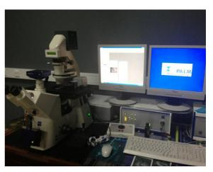
P.A.L.M. laser microdissecting microscope
