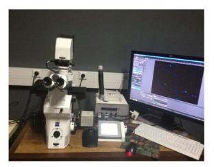
Laser scanning confocal microscope
